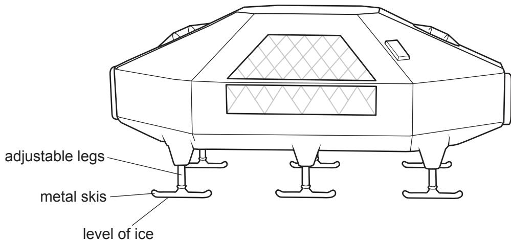
The accommodation is built on giant metal skis, with adjustable legs. Previous research stations were built on fixed legs that were buried in the ice sheet.
