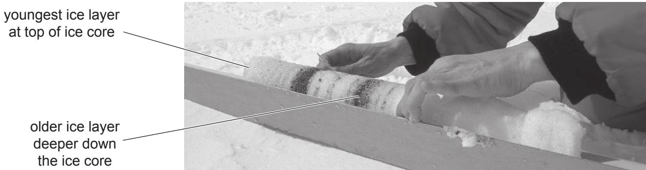
(a) Ice cores are cut into thin slices and each slice is analysed to investigate the climate in the past.
